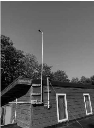
Figure 1. Placement of the ultrasonic AR125EXT microphone (Binary Acoustic Technology, Tucson, AZ) located on the roof of the Hawk Mountain Sanctuary Nature Center located along the Kittatinny Mountain Ridge in Kempton, Pennsylvania.
